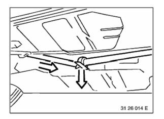
Pull propeller shaft downwards at center bearing and in so doing detach from centering pin on manual transmission or constant-velocity joint from final drive.
