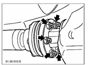
Remove constant-velocity joint from final drive.
